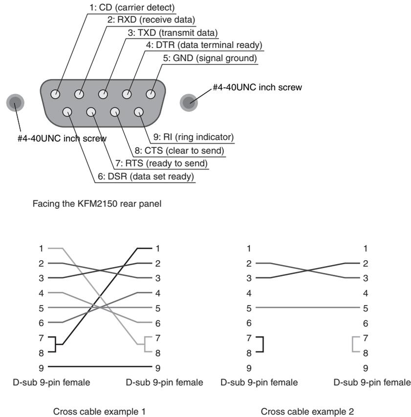
Fig. 2-17 9-pin AT type connector
