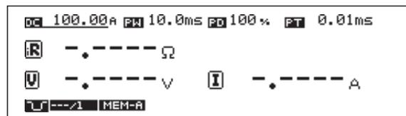
Fig. 5-11 Setup display of the current interrupt method
