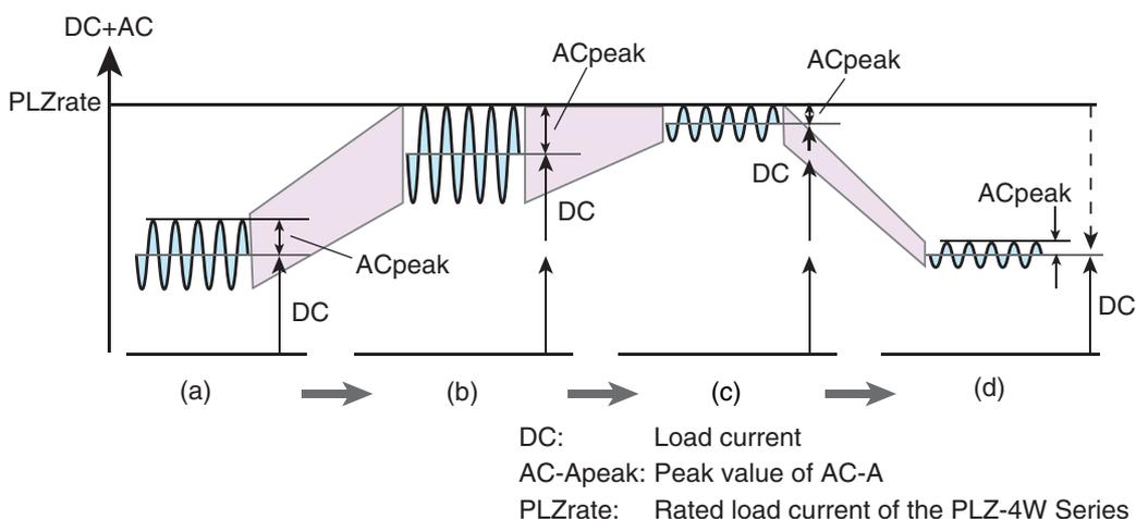
Fig. 5-10 Relationship between the measuring AC current and load current
