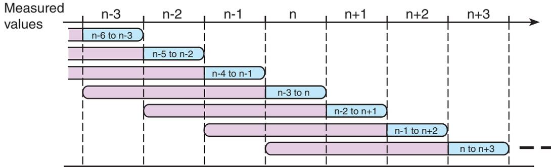
Voltmeter and ammeter cycle
