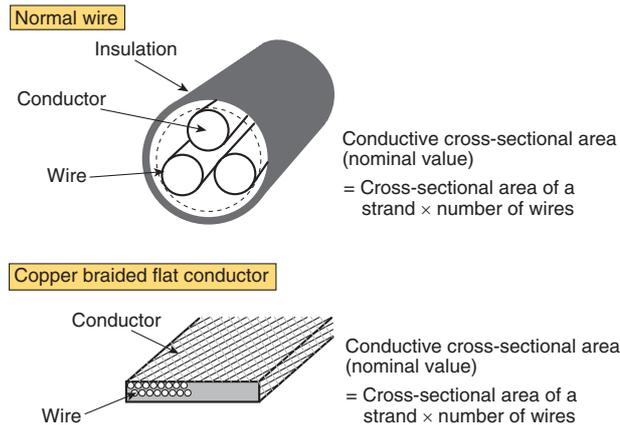
Fig. A-7 Wire structure and conductive cross-sectional area
