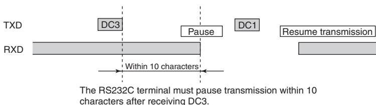
Fig. 4-17 RS232C terminal and transmission control of the KFM2150
