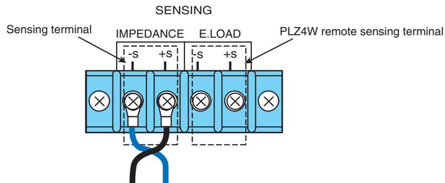
Fig. 3-6 PLZ4W remote sensing terminal (SENSING/E.LOAD)
