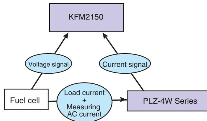
Fig. 5-3 Overview of the functional assignments
