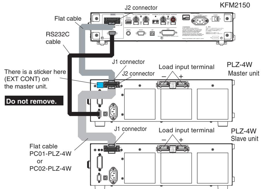
Fig. 2-14 When using two electronic load units
