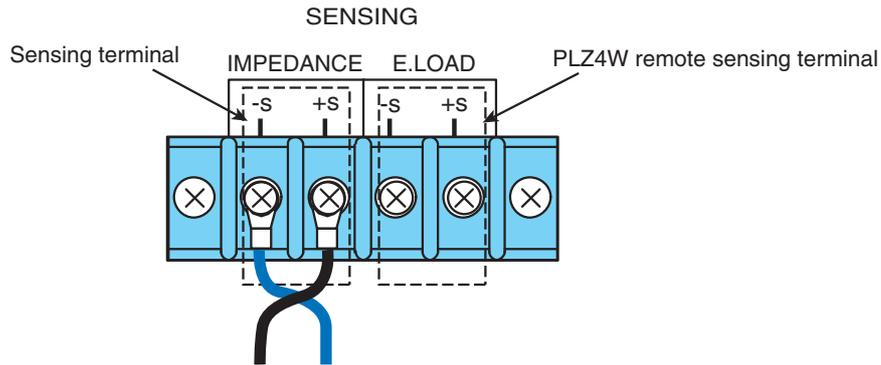
Fig. 3-9 Sensing terminal (SENSING/IMPEDANCE)
