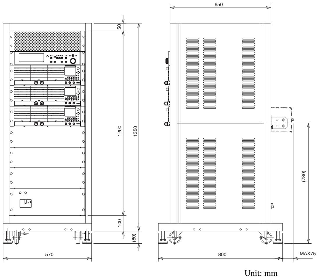
Fig. 7-7 KFM2150 SYSTEM1980-03A, KFM2150 SYSTEM2640-04A, and KFM2150 SYSTEM3300-05A outline drawings
