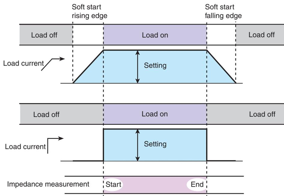
Fig. 5-5 Load current state
