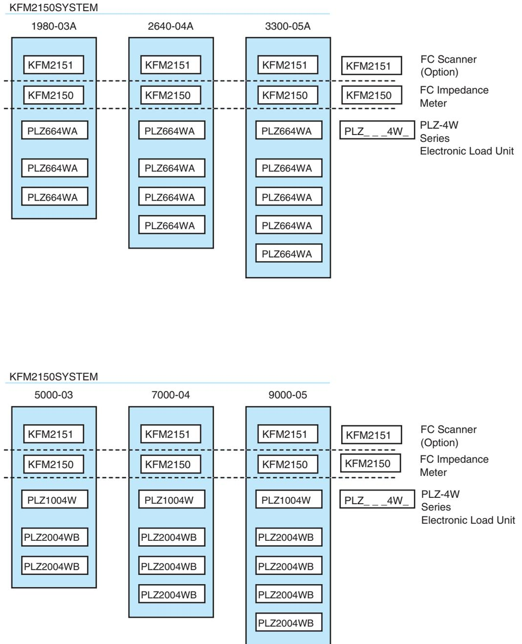
Fig. 1-4 Component instruments of the rack mount type
