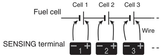
Fig. 2-11 Wiring the SENSING terminal
