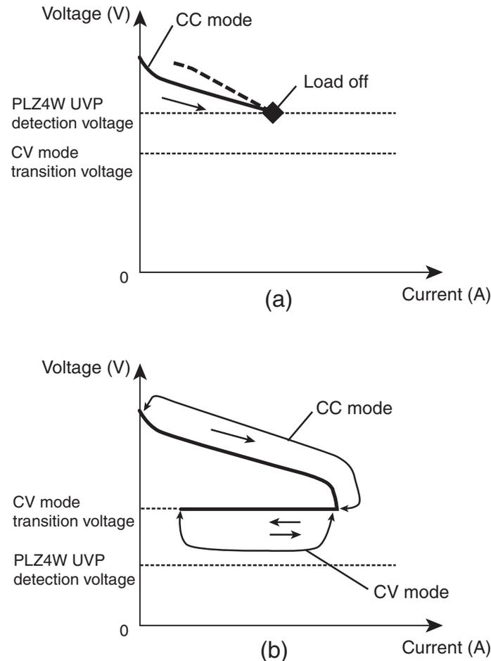
Fig. 4-12 PLZ4W UVP and CV mode transition voltage
