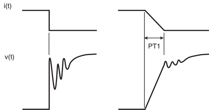
Fig. A-21 Pulse transition time PT1 and ringing
