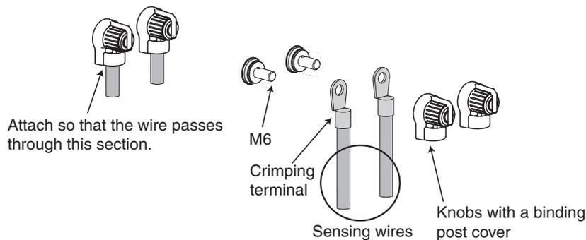
Fig. 2-8 Connecting the sensing wires for channel 1
