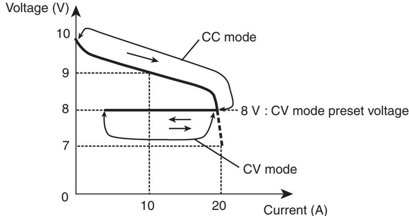
Fig. 4-11 Transition from CC mode to CV mode
