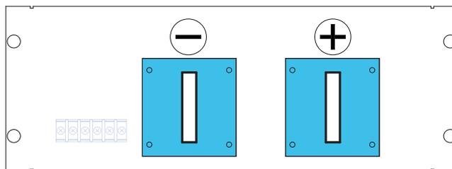
Fig. 3-4 Load input terminal
