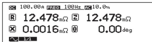
Fig. 5-7 Setup display of the AC impedance method
