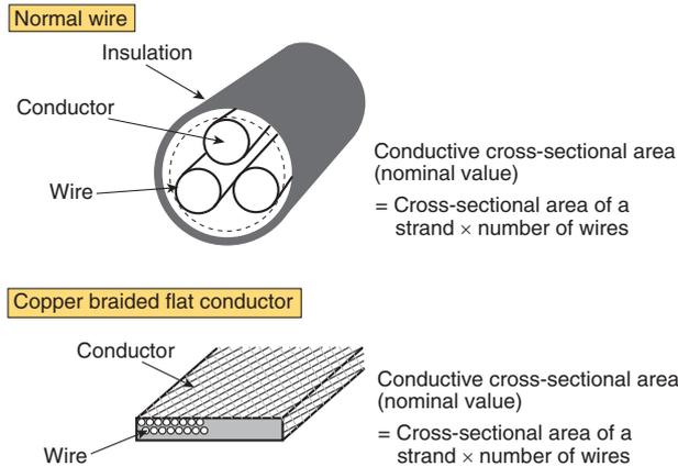
Fig. 3-3 Structure of the recommended load wire
