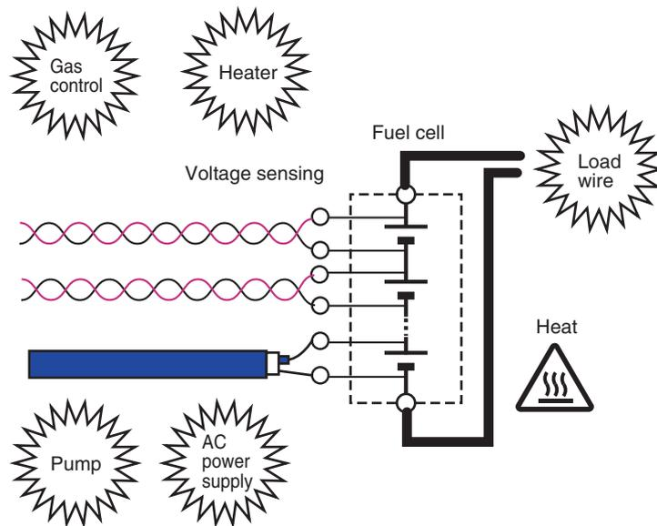
Fig. A-10 Sensing wire environment
