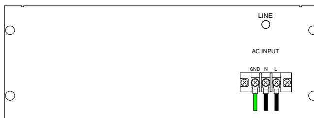
Fig. 3-14 Connecting the power cable
