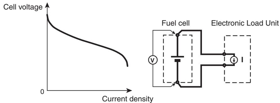
Fig. 5-1 Current and voltage characteristics
