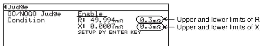
Fig. 5-22 Setting the upper and lower limits (AC impedance method)
