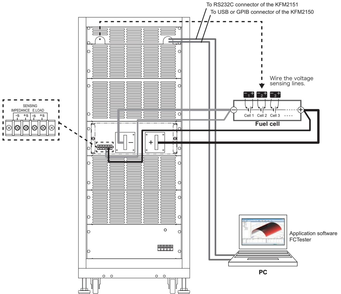
Fig. 3-2 Example of rack mount type scanner system wiring
