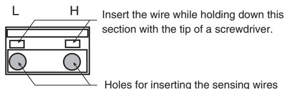
Fig. 2-9 Connecting the sensing wires for channel 2
