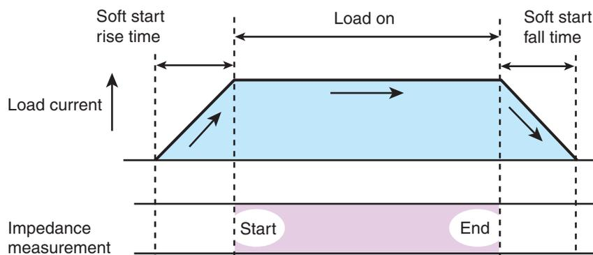
Fig. 5-2 Measurement and the operating status of the fuel cell
