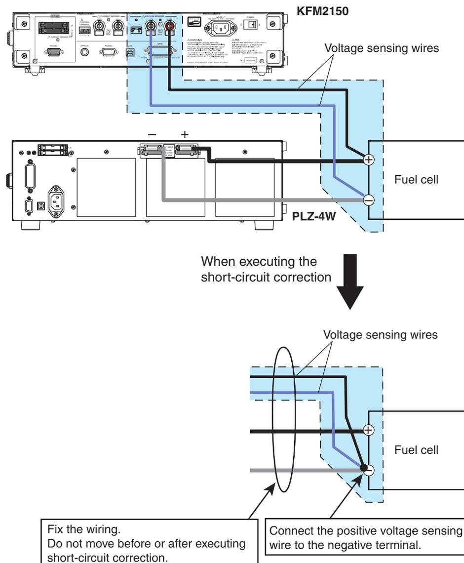
Fig. 5-19 Shorting the voltage sensing wires
