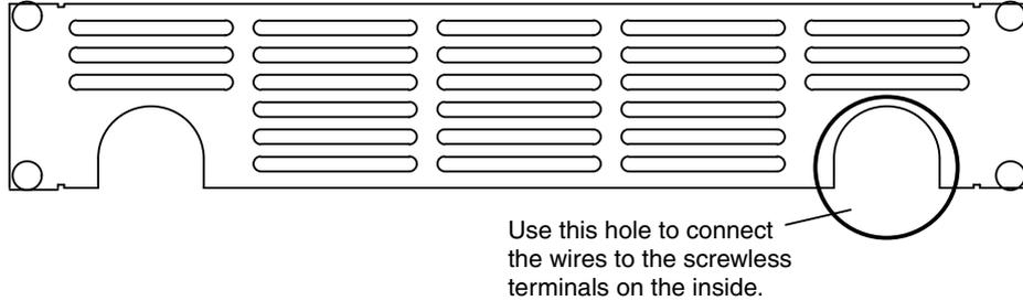
Fig. 3-10 Rear panel of where the FC scanner installed
