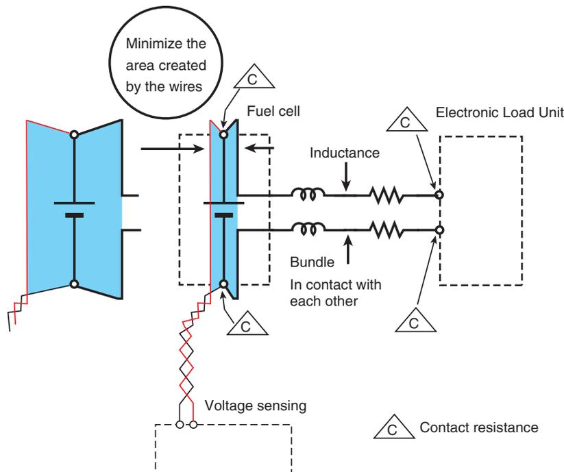
Fig. A-9 Minimum area wiring and wires in contact with each other
