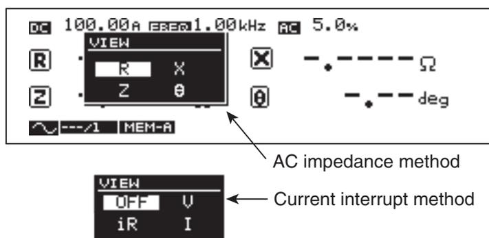
Fig. 5-16 Display setup window
