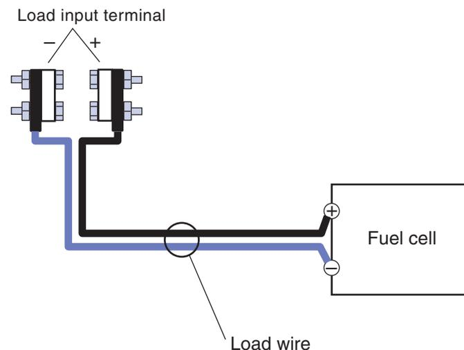
Fig. 3-5 Wires in contact with each other
