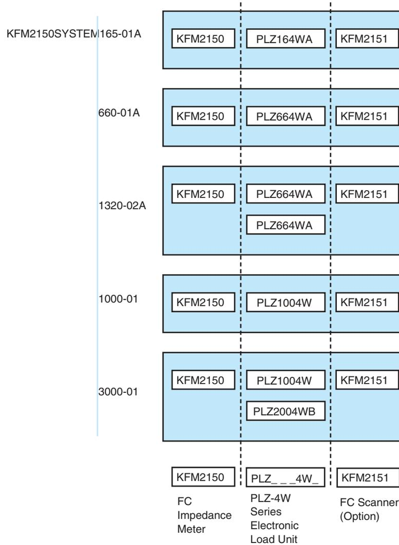
Fig. 1-3 Component instruments of the bench top type
