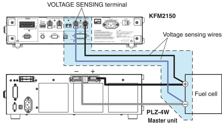
Fig. 2-10 Wiring the voltage sensing wires (channel 1 example)
