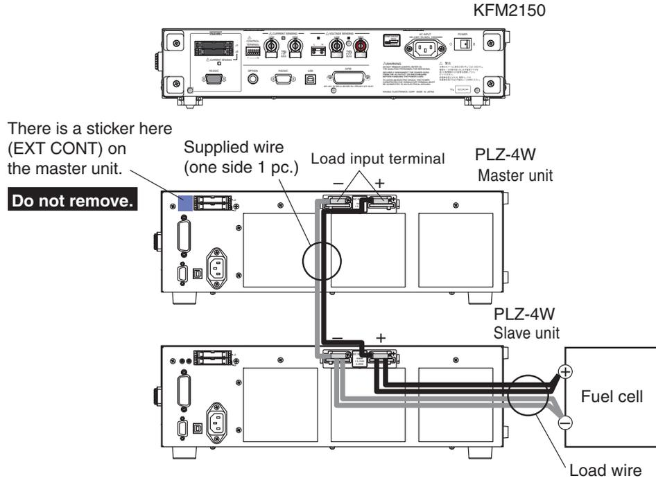
Fig. 2-5 When using two electronic load units
