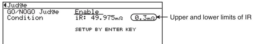
Fig. 5-23 Setting the upper and lower limits (current interrupt method)
