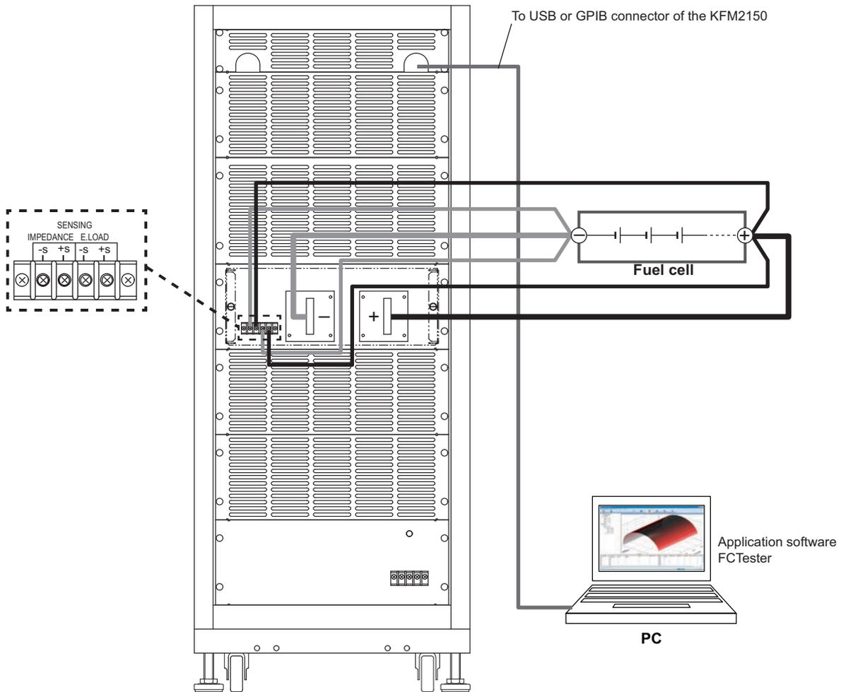
Fig.3-1 Example of rack mount type basic system wiring
