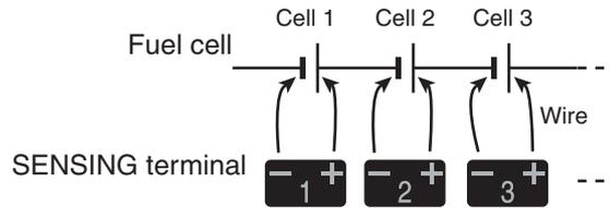
Fig. 3-11 Wiring the SENSING terminal
