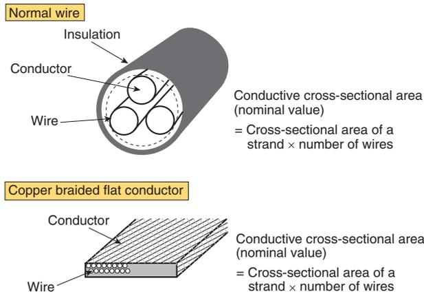
Fig. 2-3 Structure of the recommended load wire
