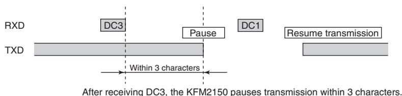
Transmission control from the KFM2150 to the RS232C terminal
