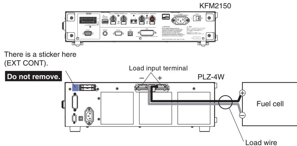
Fig. 2-4 When using one electronic load unit
