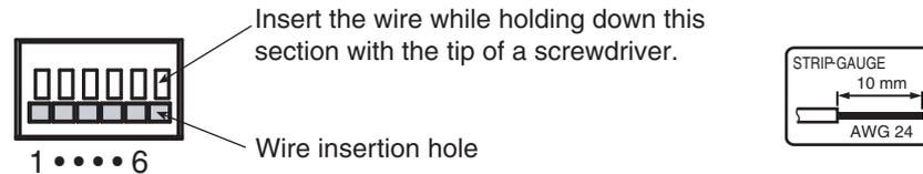
Fig. A-2 Screwless terminals and wires used
