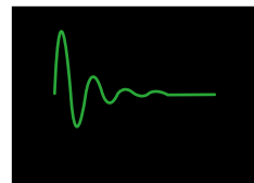
Second order impulse response (damping coefficient 0.2)
