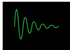
Second order impulse response (damping coefficient 0.1)
