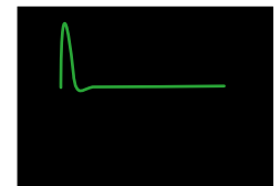
Second order impulse response (damping coefficient 0.7)
