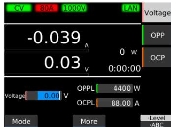
**3** Use the numeric keypad or the rotary knob to enter the voltage value.
