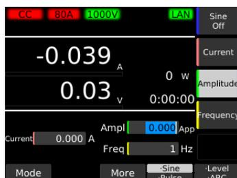
**5** Use the numeric keypad or the rotary knob to enter the sine amplitude (Amplitude).
