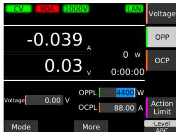
**3** Use the numeric keypad or the rotary knob to enter the power value.
