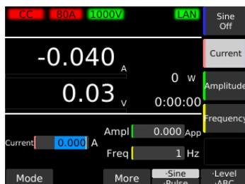
**3** Use the numeric keypad or the rotary knob to enter the load value (Current).
