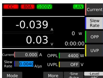
**3** Use the numeric keypad or the rotary knob to enter the slew rate value.
