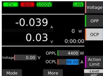
**3** Use the numeric keypad or the rotary knob to enter the current value.
