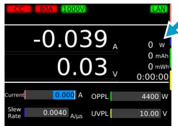
Display example of integrated current, integrated power, and elapsed time
