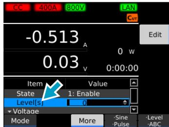
**5** Use the numeric keypad or the rotary knob to enter the value for activating the cut-off, and then press ENTER.
