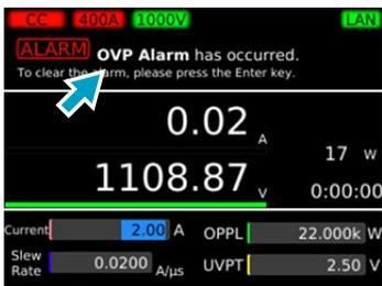
If a voltage exceeding 1100 V is applied to the DC INPUT terminals, a beeping sound is generated and an OVP alarm (overvoltage detection) appears.
