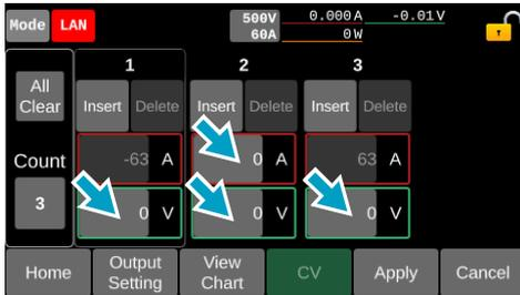
After input, the current in the case of CV mode and the voltage in the case of CC mode are sorted in ascending order from left to right at the following timings:
