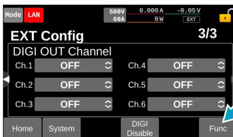
“Func” switches to “Polarity” to display the polarity setup screen for each channel.
