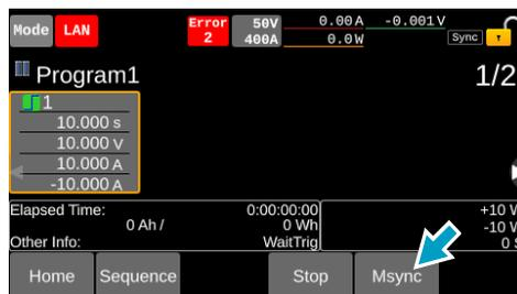
Trigger wait is released for all PXB series to be synchronized, and sequence starts simultaneously.
