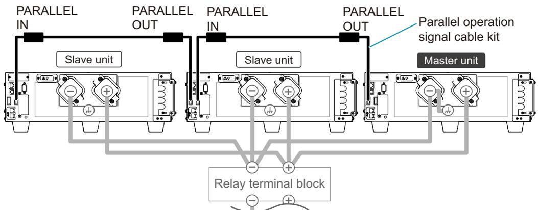
**4 Turn on the POWER switch of all PXB series units within 20 seconds.**
