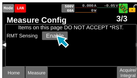
When remote sensing is enabled, the sensing icon (
