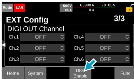
Enable the digital input/output.
