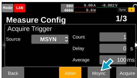
Measurement starts simultaneously on all synchronized PXB series products.
