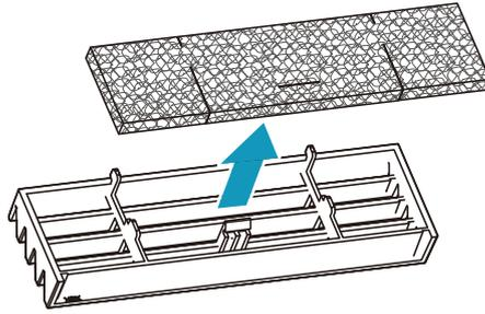
**4** Remove the dust filters set inside the front panel.
