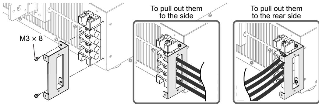
**5 Attach the rear-panel INPUT terminal cover.**
