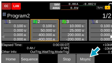
Trigger wait is released for all PXB series to be synchronized, and sequence resumes simultaneously.
