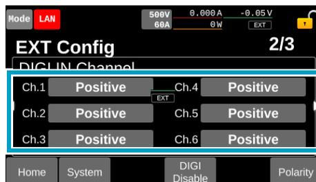
If the input field is grayed out, press DIGI Enable to enable the digital input/output.
