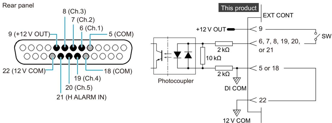
**NOTE** Since the digital input terminals are compatible with both positive and negative common, you can also set 6, 7, 8, 19, 20, or 21 to DI\_COM.
