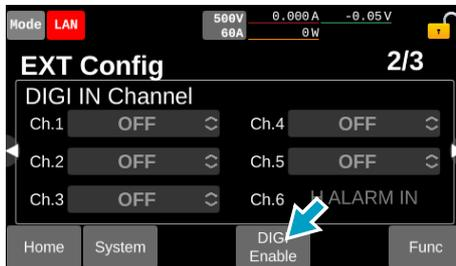
Enable the digital input/output.
