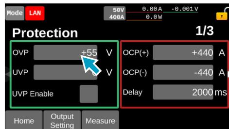
**3** Use the display or the rotary knob to enter the voltage value.
