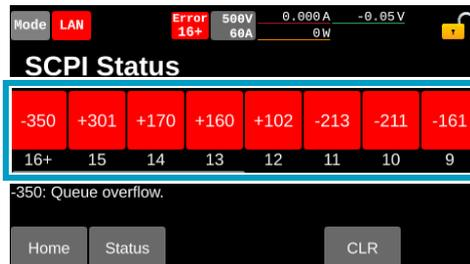
The details of the error will be displayed under the error number. The details of the error will be displayed. For details on errors, see the Communication Interface Manual on the included CD-ROM.
