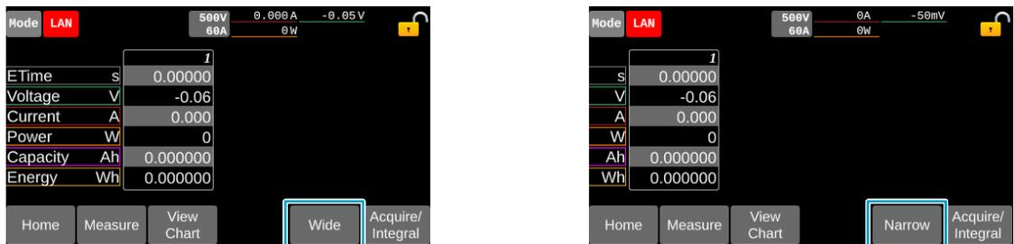
Switching between detailed and simplified displays
