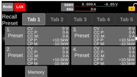
In this screen, 4 preset memories are displayed. To display other memories, press Tab at the top. Press Preset memory to recall the memory in fewer steps.
