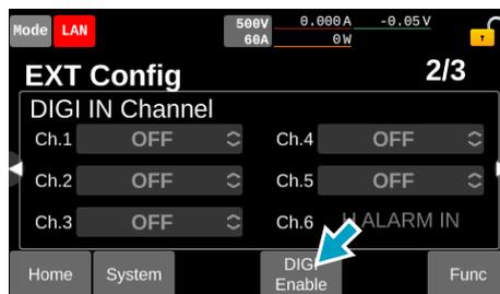
Enable the digital input/output.
