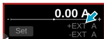
Due to Setting the Output Mode (p. 32), the values cannot be changed from the display during external control (EXT), pulse function operation (PULSE), sine function operation (SINE), or I-V characteristic function operation (I-V).
