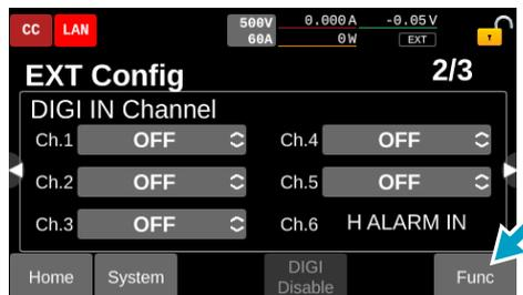
It switches in the order of “Func” → “Filter” → “Polarity” to display the polarity setup screen for each channel.
