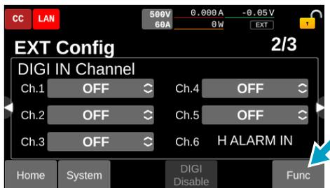
“Func” switches to “Filter,” and the filter setup screen for each channel is displayed.
