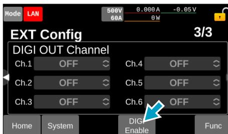
Enable the digital input/output.
