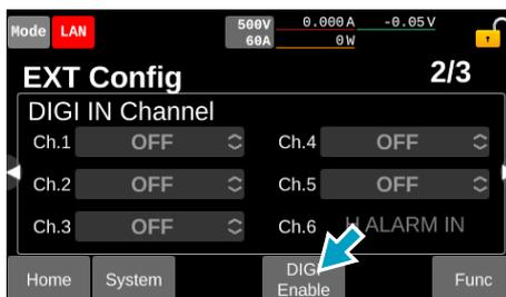
Enable the digital input/output.
